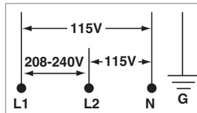
\*Note: Electrical supply service must be a 3-wire plus ground for connection as shown.
